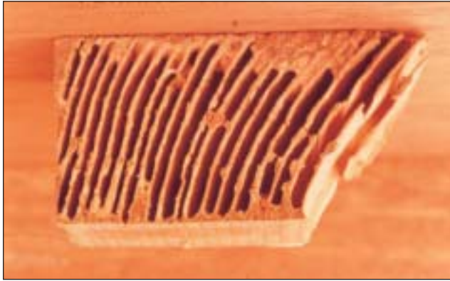
Figure 5. Typical wood damage by subterranean termites.
